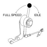
Figure 8. Speed Control Lever
