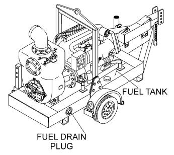
Figure 17. Fuel Tank/Drain Plug
