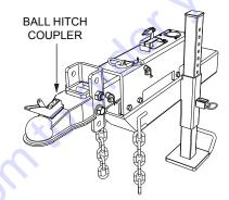
Figure C. Ball Hitch Coupler
