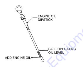
Figure 11. Engine Oil Dipstick
