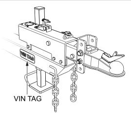
Figure B. Typical VIN Tag Location
