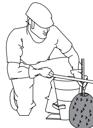
Figure S. Slump Test (Measurement)
