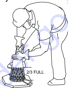
Figure O. Slump Test (2/3 Full)
