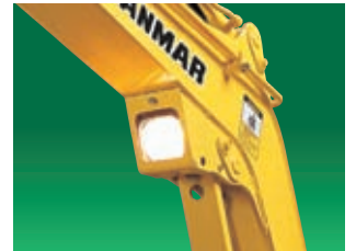
Integrated boom-light is protected from damage.
