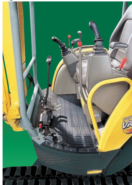
Canopy models allow entry and exit from either side.
