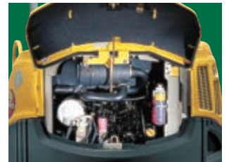
Large opening rear hood for easier maintenance.
