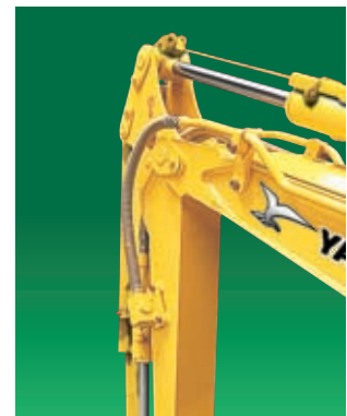
To enable the use of additional hydraulic attachments, PTO is piped to the end of the arm.
