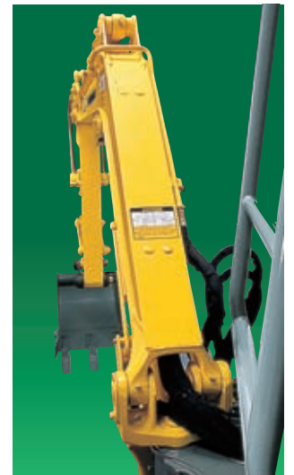
To prevent damage to the hydraulic hoses, they are housed in the inner boom for safety.
