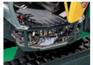
Removable side frame cover and side weight for easier maintenance.
