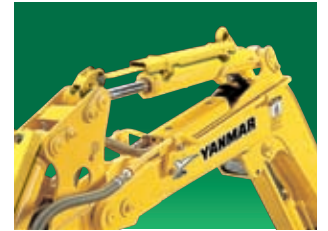
The hydraulic oil hose cover protects the hydraulic hoses from damage.
