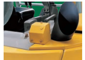
The audible traveling alarm signals people nearby when the machine is being moved.
