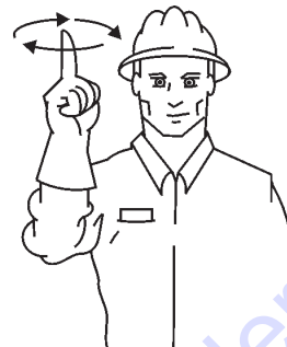
START PUMP SPEED UP
