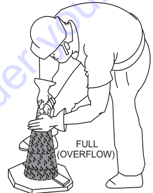
Figure 38-C. Slump Test (Full-Overflow)
