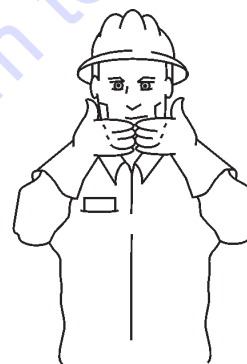
ALL DONE CLEAN-UP
