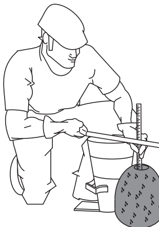
Figure 41-F. Slump Test (Measurement)
