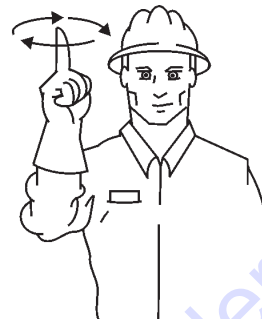
START PUMP SPEED UP
