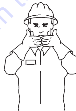
ALL DONE CLEAN-UP
