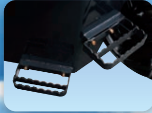
Two-stage step for safe mounting/dismounting
