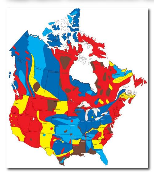
This aggregate map is not intended, nor shall it be used, to precisely define all aggregate in a given area. Instead it is published as a "general guide" to the predominant aggregate hardness (as it relates to grinding) likely to be encountered in the area defined by the various colors.
