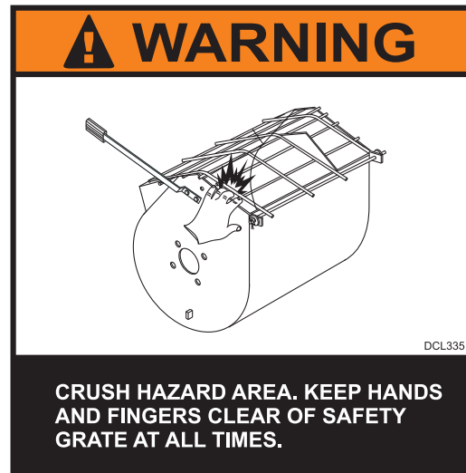
Figure 37. Safety Grate (Crush Hazard)
