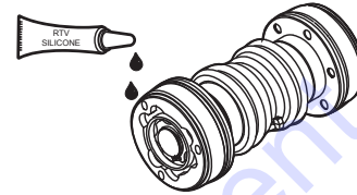
Figure 37. Applying RVT Silicone
