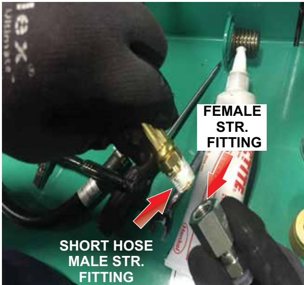
Figure 26. Straight Fitting Connection
