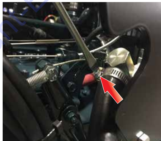
Figure 10. Loosen Hose Clamps
