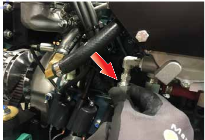
Figure 29. Connect Hose to Fitting
