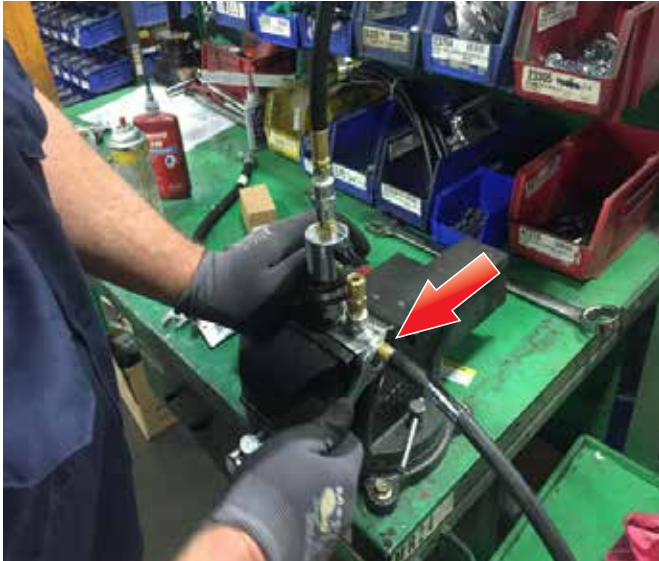
Figure 22. Old Hoses Removal
