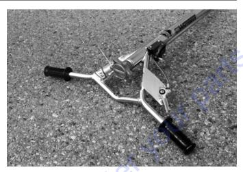
Remove one brass nut from the cable end. Thread the second brass nut towards the cable as far as possible. Insert the cable end into yoke as shown in the QUICK PITCH installation. Replace the brass set nut on the cable end. Tighten the set nut by finger as far as possible to remove slack from the cable. Using a wrench, tighten the locking nut on the other side of the boss to lock the cable in place.
