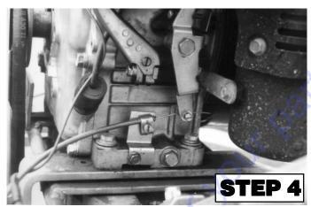
Connect the throttle cable to the engine. Keep in mind there should be a piece of wire installed on the machine to show you where to route the throttle cable. When connecting the cable housing, make sure that no more than 1/4" (6.4mm) of the cable housing protrudes past the housing clamp on the engine (Step 4). After the cable has been installed on the engine, tighten the clamp on the throttle control, operator position of the handle to lock the throttle cable at the proper length.
