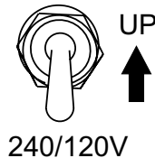
Figure 22. Full Power Switch 120V Position (Up)
