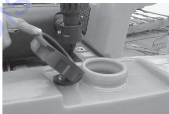
Figure 9. Checking Water Tank
