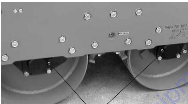
Figure 25. Vibrator Oil Maintenance
