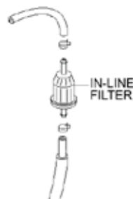
Figure 12. In-Line Fuel Filter
