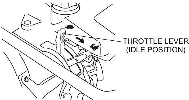
Figure 9. Throttle Lever (Idle Position)
