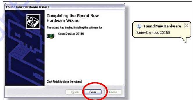
Figure 18. CAN Driver Installation Complete
