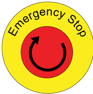
Figure 21. Emergency Stop Switch
