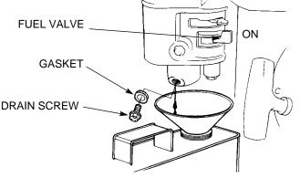
4. Reinstall the drain screw and gasket.
