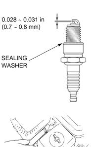
plug washer is in good condition, and thread the spark plug in by hand to prevent cross-threading.
