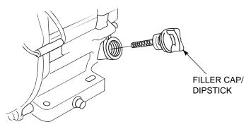
2. Insert and remove the dipstick without screwing it into the filler neck. Check the oil level shown on the dipstick.
