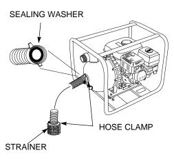
The strainer provided with the pump should always be attached to the end of the suction hose with a hose clamp as shown.
