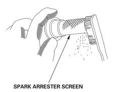
4. Install the spark arrester, muffler protector, and muffler in the reverse order of disassembly.
