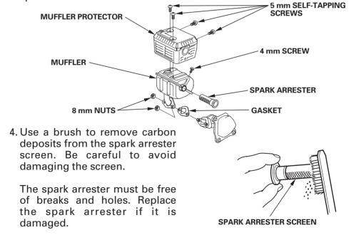
5. Install the spark arrester, muffler protector, and muffler in the reverse order of disassembly using a new gasket.
