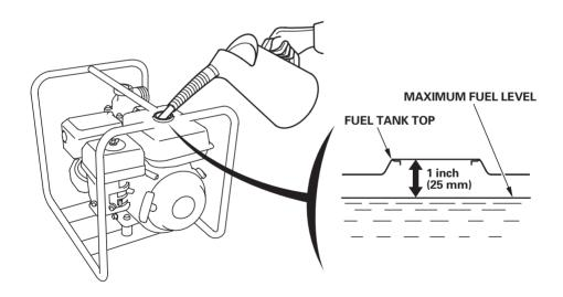
Refuel in a well-ventilated area before starting the engine. If the engine has been running, allow it to cool. Refuel carefully to avoid spilling fuel. Do not fill the fuel tank completely. Fill tank to approximately 1 inch (25 mm) below the top of the fuel tank to allow for fuel expansion. If may be necessary to lower the fuel level depending on operating conditions.
