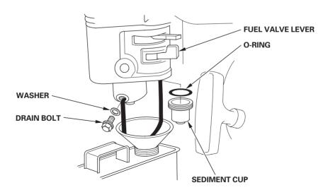
3. After all the fuel has drained into the container, reinstall the drain bolt and sediment cup. Tighten them securely.
