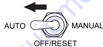
Figure 57. Auto Start/Stop Switch (Auto Position)
