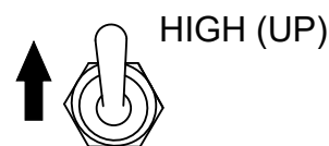
Figure 46. Engine Speed Switch (High Position)
