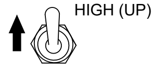
Figure 56. Engine Speed Switch (High Position)
