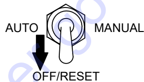
Figure 60. Auto Start/Stop Switch (Off/Reset Position)
