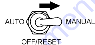
Figure 30. Auto-Off/Reset Manual Switch (Manual Position)
