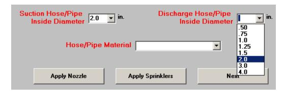
The inside diameter of the suction hose/pipe is especially important because excessive dynamic suction head can cause the pump to cavitate. Cavitation will result in poor pump performance and possibly damage to the pump. To avoid cavitation, the inside diameter of the suction hose/pipe should be as large as possible. Ideally, the suction hose/pipe should be no smaller than the pump's suction port diameter.
