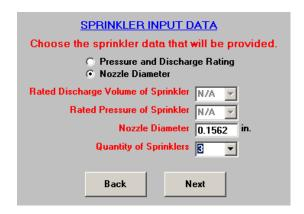
The sprinkler nozzle diameter is the diameter of the orifice where the water exits the sprinkler. This value is sometimes stamped on the nozzle and can only be entered for sprinklers with a single nozzle.
