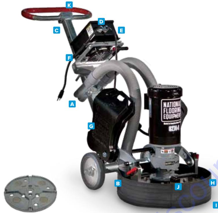
Magnetic tooling easily snaps into place
