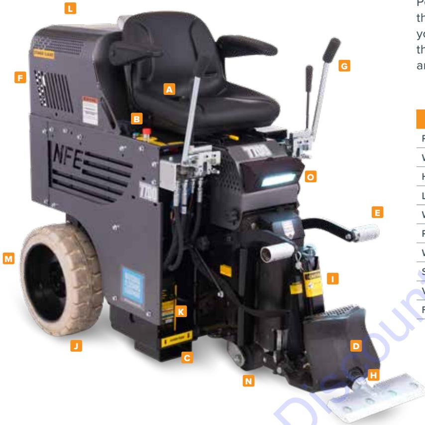
Powered by 12 200-amp hour batteries that exceed the industry standard, this machine is everything you need it to be. Bigger, heavier, and faster than the 5700, it is designed to remove difficult material and built to operate on almost any jobsite.
