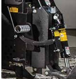
Adjust the height of the slide plate using the hydraulic hand control for precise angling. Comes standard on **7700** and **8000** ride-on scrapers
