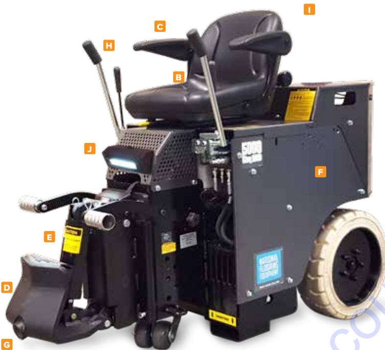
The 5000 is a compact, ride-on floor scraper designed with a low-profile frame that increases ease of transport and maneuverability on the job.
