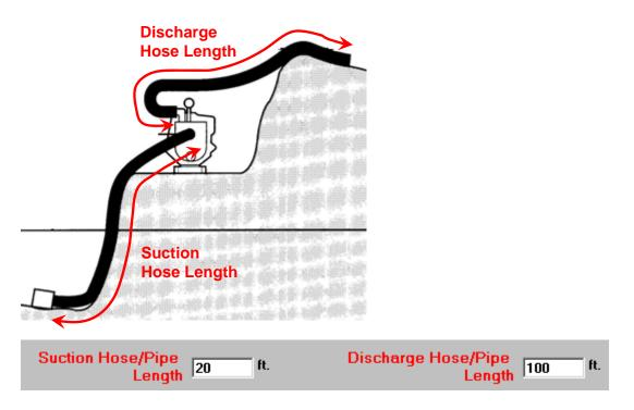
Like the inside diameter, the length of the suction hose/pipe is especially important. Using a very long suction hose/pipe can result in excessive suction head loss and possible cavitation. To avoid cavitation, the suction hose/pipe should be as short as possible.
