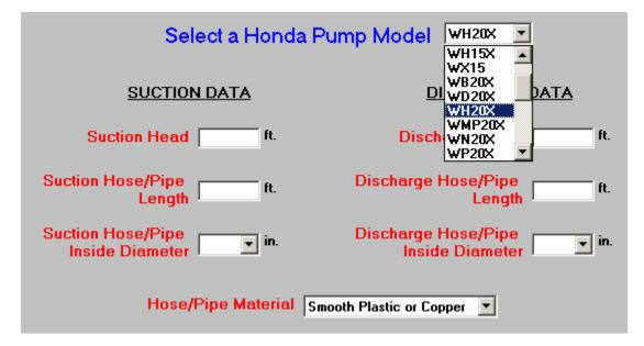
If you are considering a pump where high pressure and low discharge volume are needed, which is usually the case when using sprinklers or a nozzle, you should select a WH series (high-pressure) pump. However, if discharge volume is the major concern, a WB or WT series may be preferred. A WSP pump can be chosen if an electric submersible pump is preferred.
