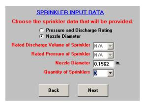
The sprinkler nozzle diameter is the diameter of the orifice where the water exits the sprinkler. This value is sometimes stamped on the nozzle and can only be entered for sprinklers with a single nozzle.
