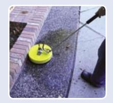
Connect to lance using q/c fittings on the lance and whirl-a-way. Ensure the M22 hose is connected properly before use.
