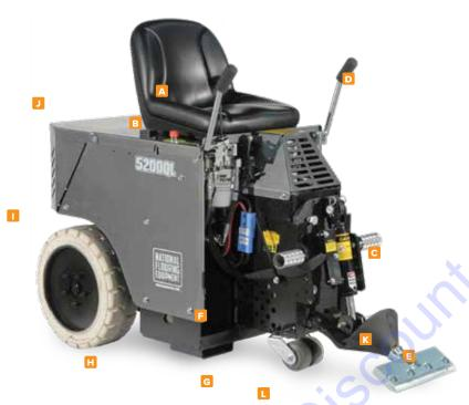
The 5200QL is designed for jobs that require continuous operation, and it offers the only slide-out replaceable battery in the industry with a rear-accessed battery pack that is easily installed, changed, and transported. With no belts or gears, this scraper boasts low maintenance costs while maximizing production. Great for commercial surface removal and preparation it is quiet and compact enough for residential jobs.
