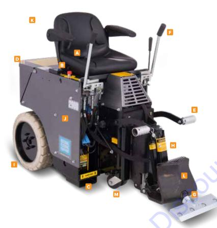
Designed specifically for high-speed soft goods removal, this machine is a durable, emission-free, budget-concious workhorse. The 2900 will remove VCT and other soft and hard goods quickly and efficiently for time sensitive applications.
