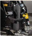
Adjust the height of the slide plate using the hydraulic hand control for precise angling. Comes standard on **7700** and **8000** ride-on scrapers
