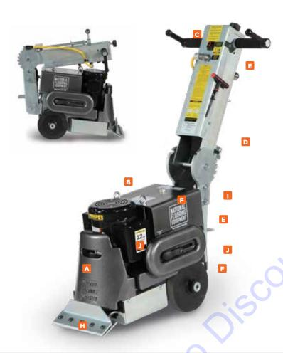
The Commander removes the worst of today's soft goods, such as glued-down floors, gummy commercial carpet, VCT, sheet vinyl, rubber tile, linoleum, indoor and outdoor sport surfaces, roofing material, and more.
