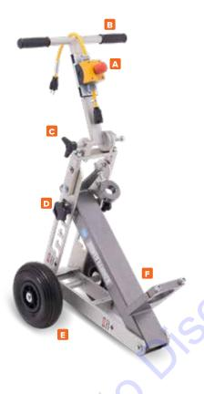
Give your hands and back a break and let the Power Hammer Trolley make you faster, more efficient, and productive. This machine works as a floor stripper and scraper on concrete and wood surfaces. Great for removal of epoxy, ceramic tile, vinyl, VCT, cork, adhesives, mastic, and more. The Power Hammer Trolley is perfect for rock breaking and block demolition. Hammer sold separately.
