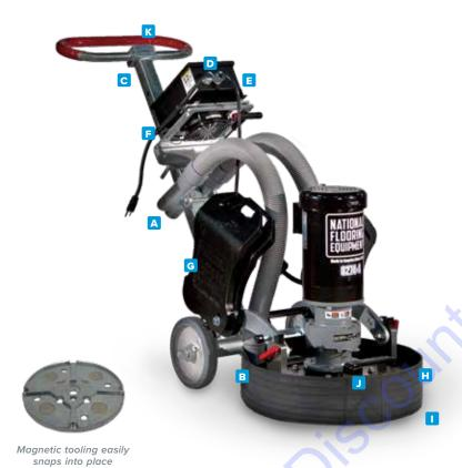
The 8274-4 is the only grinder on the market offering 3 HP at 115 volts while operating at a 230-volt level. With variable speed and a soft start to control its amperage draw, the 8274-4 adjusts to the needs of small or large jobs. This machine is well suited for removal of thin-set, coatings, adhesive, prepping concrete for overlays or coatings, and polishing.
