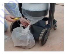
> Pull down a length of new bag from the chamber, until it reaches the bottom support plate
