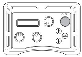
2 Set the feeding flow on the unit to max by turning the control on the remote control clockwise.
