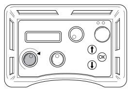
3 Tension the wire by carefully turning the knob on the pressure reduction block clockwise until the wire is tensioned sufficiently. Make sure to always check that the wire is seated correctly in all the wheels on the saw.
