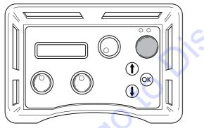
2 Turn the controls for blade rotation and water coolant to their maximum positions to start blade rotation and the water coolant.
