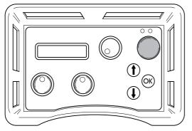
2 Set the feeding flow on the unit to max by turning the control on the remote control clockwise.
