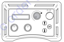
5 Carefully increase the motor speed by turning the control for motor rotation. A suitable working pressure when cutting usually lies between 100 and 130 bar, but varies depending on how many wheel sets are used in the magazine, how much wire is in use and the hardness of the material to be cut.
