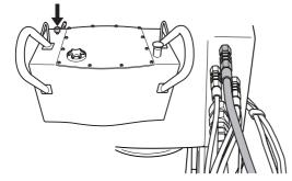
When the power cable and water hoses and hose assembly are connected, the machine can be started.
