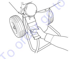
4 Connect the incoming water hose to the water coupling on the bottom of the motor front on the hydraulic unit.
