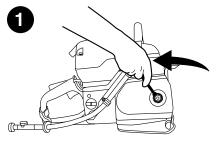
Loosen side cover nut and remove side cover.
