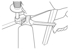
Before the machine is started, carefully check that the new bit is firmly attached.
