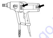
• Use compressed air to periodically clean the motor. Remove the inspection cover and clean the cover.
