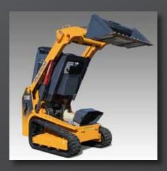
**SERVICEABILITY** is made easy with a large gas-spring assisted engine cover and tiltable ROPS/FOPS assembly. Patented tilt-out foot pod allows for best-in-class foot well cleanout and easy access to components under the cab.
