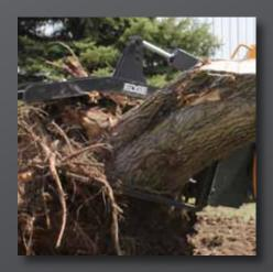
hydraulic system a pressure of 3,000 psi (207 bar) delivers high performance and fast cycke times. Lift cylinders incorporate cushioning for smoother operation when lowering the lift arm.
