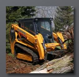
senses machine load electronically, monitoring and adjusting the hydrostatic drive pump resulting in tractive effort of 11,840 lbs. (5371 kN) on the 1750RT and 12,349 lbs. (5606 kN) on the 2100RT.
