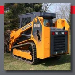
**DEDICATED**, **WELDED TRACK LOADER CHASSIS a** aids in superior weight distribution which enhances stability, grading, tractive effort and ride control.
