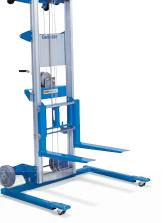
Adjustable base legs straddle loads or fixed objects up to 36 in (91 cm) wide. Perfect for lifting small pallets, appliances and other bulky objects. (GL<sup>™</sup>-4, GL<sup>™</sup>-8, GL<sup>™</sup>-10, GL<sup>™</sup>-12)
