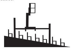
8 Install frame retaining pins at each corner of the Super-Straddle and release the tension on the winch cable. To insert frame retaining pins, align the holes and lift up on the gray tab on the pin retaining interlock box.
