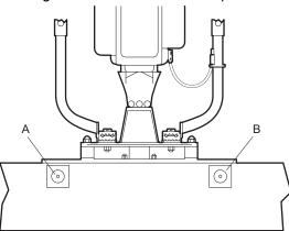
2. Set the operating handles in working position by using the lock levers.
