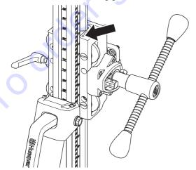
• Start with the top guide roller. Use a flat screwdriver and turn clockwise to guide the roller closer to the column.
