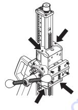
Loosen set screws holding guide roller shafts.
