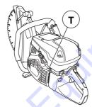
Rec. idle speed: 2700 rpm
