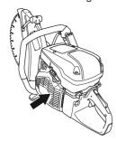
NOTICE! A dirty or blocked air intake results in the machine overheating which causes damage to the piston and cylinder.
