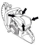
Check the air filter and replace if necessary.
