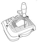
Lubricate the recoil spring with light oil. Fit the pulley and tension the recoil spring.
