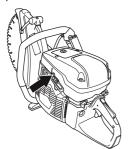
Stop switch: Make sure that the stop switch (STOP) is in the left position.
