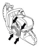
Pull the cord out about 30 cm and lift it into the cut-out in the periphery of the starter pulley. When the cord is intact: Release the spring tension by letting the pulley rotate slowly backwards.
