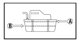
NOTE : The compressor will not operate while the drain pump is discharging in water for the Office Pro 12 and Office Pro 18.
