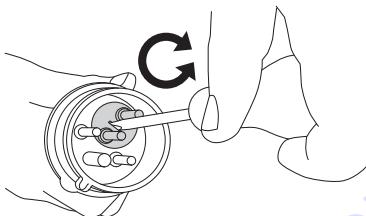
**NOTICE!** The Piranha/PCD tools are designed to run in only one direction.
