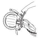
• Grip the rear handle with the right hand. When you grip the rear handle this releases the switch lock.
