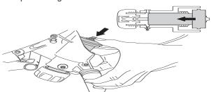
Lubricate the guide roller's sleeve using grease. Fit the grease gun on the grease nipples (A) and pump in grease until clean grease emerges from the overflow hole (B).
