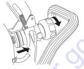
The guide roller is pressed into the knob. In order to loosen the guide roller, you need to continue turning the knob until it loosens completely.
