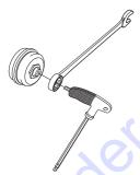
Lubricate using bearing grease inside the rollers before the new rollers are fitted.
