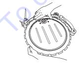
• Fit the support roller guard and ensure that the flanges on the guide rollers still enter the blade's grooves correctly. Now tighten the three screws fully.
