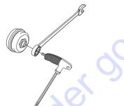
Lubricate using bearing grease inside the rollers before the new rollers are fitted.
