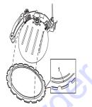
Press in the guide roller if necessary, so that it climbs into the groove on the blade.
