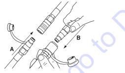
**CAUTION!** Two hose kits can be connected when hose lengths exceeding 18 m are required. Do not connect more than two kits as the couplings cause large power loss. See the Technical data.
