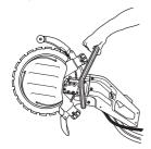
Grip the rear handle with the right hand. When you grip the rear handle this releases the switch lock.
