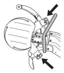
Pull out the lock for the front handle and move the handle to the service position.
