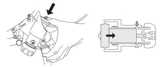
Lubricate the guide roller's sleeve using grease. Fit the grease gun on the grease nipples (A) and pump in grease until clean grease emerges from the overflow hole (B).
