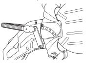
Remove the three screws holding the support roller guard using a 6 mm hex key and lift off the cover.
