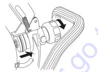
The guide roller is pressed into the knob. In order to loosen the guide roller, you need to continue turning the knob until it loosens completely.
