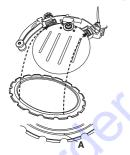
Press in the guide roller if necessary, so that it climbs into the groove on the blade.
