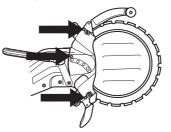
• Rotate the blade and make sure that the support rollers are not clamped against the blade.
