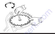
IMPORTANT! Do not forget to tighten the belt and check the belt adjustment before cutting. See the instructions under the heading "Inspecting and adjusting the drive belt".
