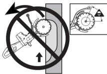
Always hold the machine in a firm grip with both hands. Hold it so that the thumbs and fingers grip round the handles.
