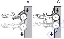
Follow the same saw cut, but further in the work piece (C), and repeat the work with the crowbar.
