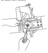
Remove the cutting arm by pulling it straight out from the machine.
