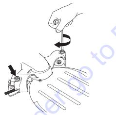
Adjust so you can easily stop the support rollers using your thumb when the blade is rotated. The support rollers should only follow the blade occasionally.
