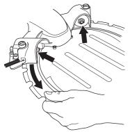
Adjust the adjuster screws so that the support rollers make contact against the blade.
