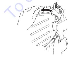
• Tighten the locking nuts on the support roller guard.
