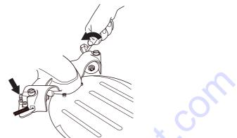
• Rotate the blade and make sure you can still hold the rollers with your thumb when the blade is rotated.
