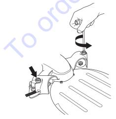
• Loosen the knob to offload the springs.
