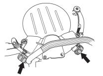
• Remove the four screws holding the support roller guard using a 6 mm hex key and lift off the cover.
