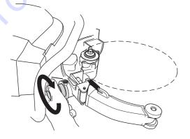
• Insert the new guide roller in the chassis. Now press the guide roller into the knob.
