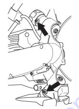
• Pump in grease until clean grease emerges from the overflow hole.
