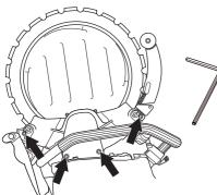
Rotate the blade and make sure that the support rollers are not clamped against the blade.
