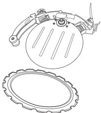
Unscrew the knob. First turn the knob a few turns until you feel a resistance. The guide roller then follows the knob out and stops when it feels a resistance.
