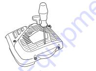
• Lubricate the recoil spring with light oil. Fit the pulley and tension the recoil spring.
