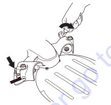
Unscrew the adjuster screws a few turns.
