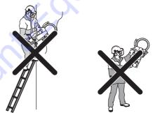
• Always hold the machine in a firm grip with both hands. Hold it so that the thumbs and fingers grip round the handles.
