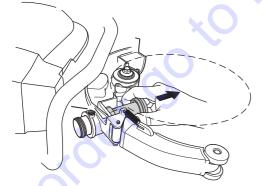
Screw the knob until it bottoms, and then loosen the knob 2 turns.
