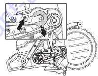
Replacing the drive belt
