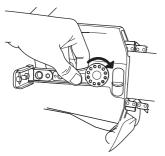
Discount. Edinoment. Cor Release the spring. Hold the bar upwards as you move the handle forward. Note that the arm's mechanical stop shall not be reached. The stop prevents the arm from pointing forwards and prevents cutting.
