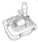
Lubricate the recoil spring with light oil. Fit the pulley and tension the recoil spring.
