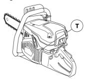
Rec. idle speed: 2700 rpm
