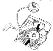
Remove the recoil spring by turning the starter over and loosen the hooks, with the help of a screwdriver. The hooks hold the return spring assembly on the starter.
