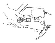
Press the spring down on the chain tensioner handle.
