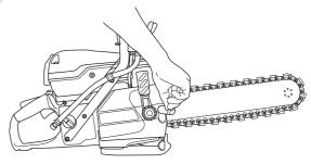
A correctly tightened chain should be easy to pull around by
