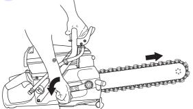
· Hold the bar upwards as you move the handle forward.
