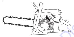
Stop switch: Make sure that the stop switch (STOP) is in the left position.
